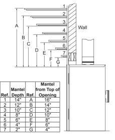
Figure 6 - Clearances for Combustible Mantels
